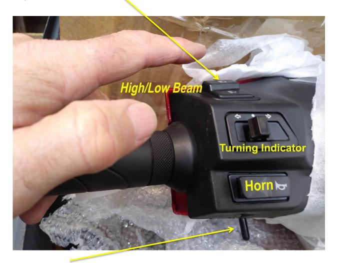
Brake Lock Rod: While squeezing left brake, push rod up to lock. Squeeze brake to release. Will prevent scooter from rolling on hill when parked.
